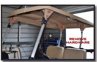
Remove lower strut bolts and remove rear struts. If installing a seat on a Yamaha G-22, retain rear struts for later use.
