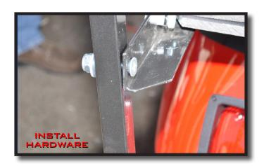
Reinstall front seat backs using hardware retained in step 3.
