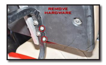
Remove OEM front seat backs. Retain hardware.
