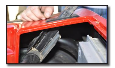
Insert **Main Brackets** into holes where OEM front seat supports were removed. Be sure the tabs are pointed to the cart's CENTER, as shown. Secure the **Main Brackets** with hardware retained in step 6.
