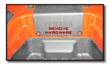
Remove OEM front seat supports. Retain hardware.
